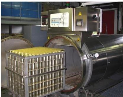
*Highest requirements: Polystone® P SSAG layer pads must stand high temperature, pressure and steam in autoclaves used for the food sterilization process*
